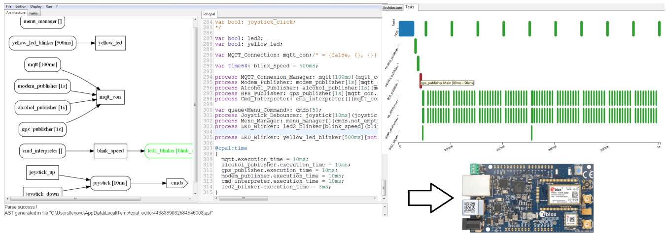
Fig. 2. CPAL model of the application. The left-hand side is the view of the functional architecture with the functions and the data flows making up the application. The CPAL code is in the center. The right-hand side shows a Gantt chart of the activation of the tasks implementing the application. This model can be executed on a workstation and without any changes interpreted (Bare-Machine Model Interpretation) on the ARM mbed Cortex M3 processor of the U-Blox C027 IoT board.
