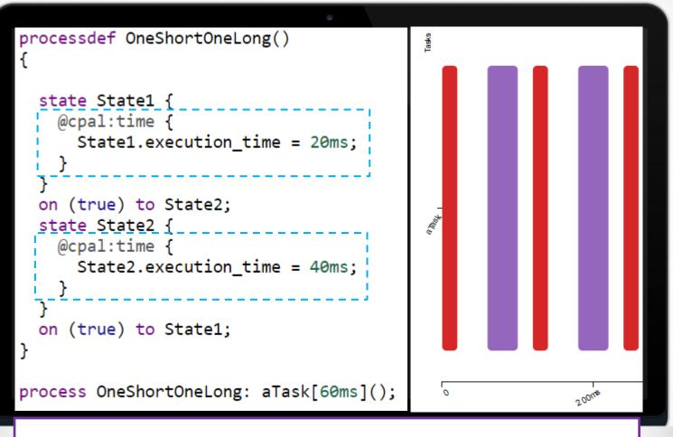
**Timing annotations** can be derived by built-in monitoring facilities and are respected by the simulator
